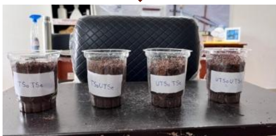
Figure 6: 4 Plastic cups - 2 with silicea treated soil; 2 with untreated soil
